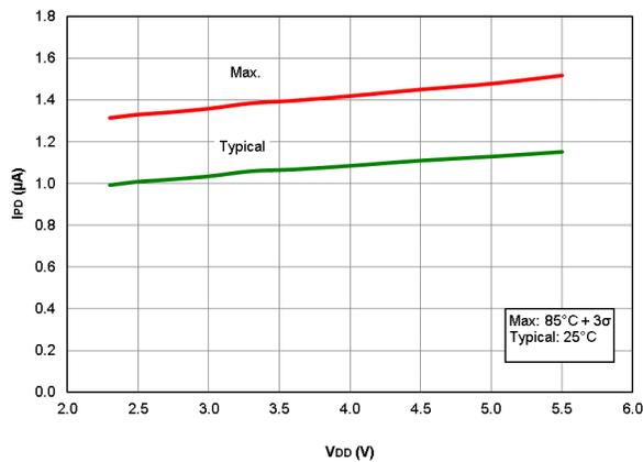
**Figure 40-4.  $I_{PD}$  Fixed Voltage Reference (FVR), PIC16LF18426/46 only**
