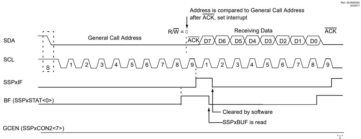
In 10-bit Address mode, the UA bit will not be set on the reception of the general call address. The client will prepare to receive the second byte as data, just as it would in 7-bit mode.
