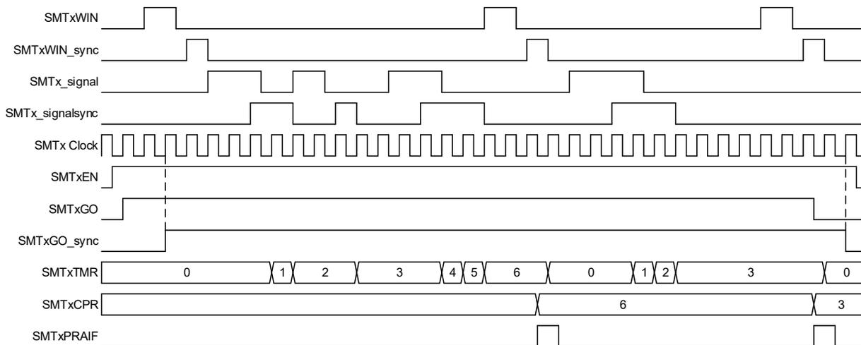
**Figure 21-12. Gated Windowed Measurement Mode, Single Acquisition Timing Diagram**
