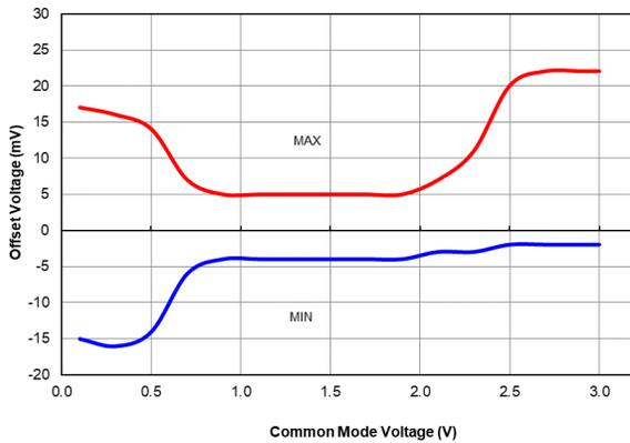
**Figure 40-80. Comparator Hysteresis, Normal Power Mode (CxSP = 1), V<sub>DD</sub> = 5.5V, Typical Measured Values, PIC16F18426/46 only**
