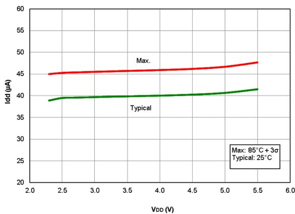
**Figure 40-6.  $I_{PD}$  Brown-Out Reset (BOR), BORV = 1, PIC16LF18426/46 only**
