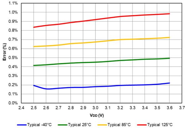
**Figure 40-92. FVR Voltage Error 1x, PIC16F18426/46 only**
