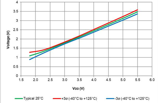
**Figure 40-97. Schmitt Trigger Low Values, All devices**
