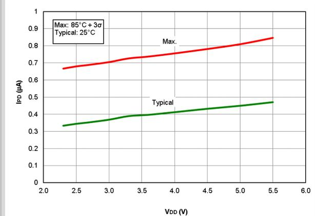
**Figure 40-13.  $I_{DD}$  XT Oscillator 4 MHz, PIC16LF18426/46 only**
