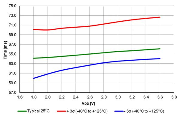
**Figure 40-108. Wake from Sleep, VREGPM = 0, HFINTOSC = 4 MHz, PIC16F18426/46 only**
