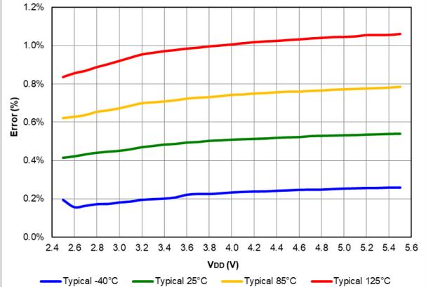
**Figure 40-93. FVR Voltage Error 2x, PIC16LF18426/46 only**
