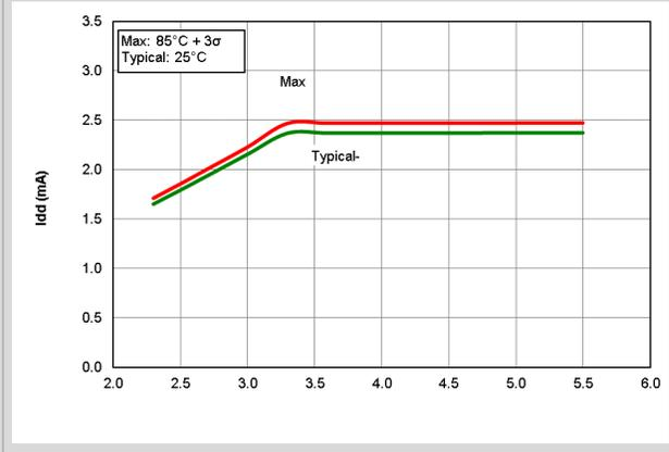
**Figure 40-21.  $I_{DD}$  HFINTOSC Idle Mode,  $F_{OSC} = 16$  MHz, PIC16LF18426/46 only**
