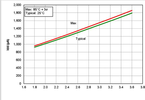
**Figure 40-24.  $I_{DD}$  HFINTOSC Doze Mode,  $F_{OSC} = 16$  MHz, PIC16F18426/46 only**
