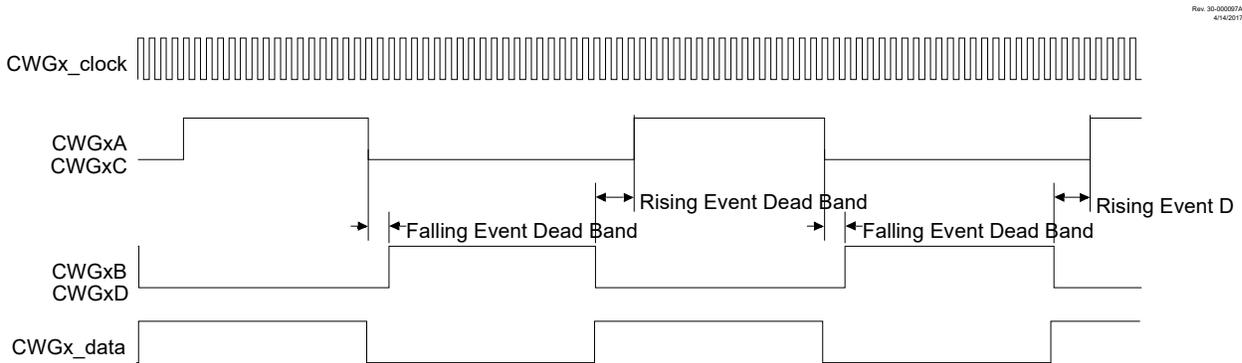
**Note:** CWGx\_rising\_src = CCP1\_out, CWGx\_falling\_src = ~CCP1\_out
