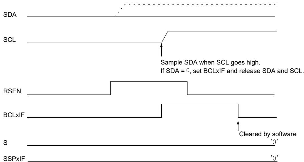
If SCL goes from high-to-low before the BRG times out and SDA has not already been asserted, a bus collision occurs. In this case, another host is attempting to transmit a data '1' during the Repeated Start condition, see [Figure 29-37](#).
