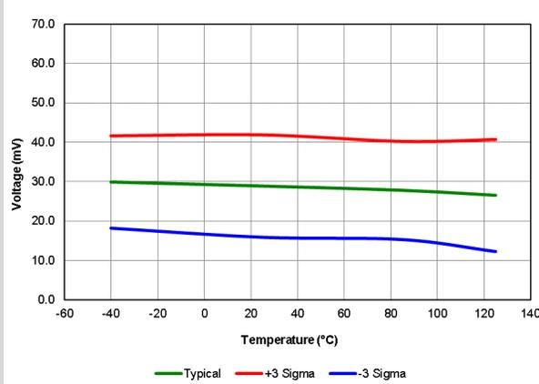
**Figure 40-40. Brown-Out Reset Voltage, Trip Point BORV = 01, PIC16LF18426/46 only**
