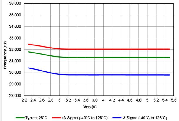
**Figure 40-27. HFINTOSC Typical Frequency Error, PIC16LF18426/46 only**
