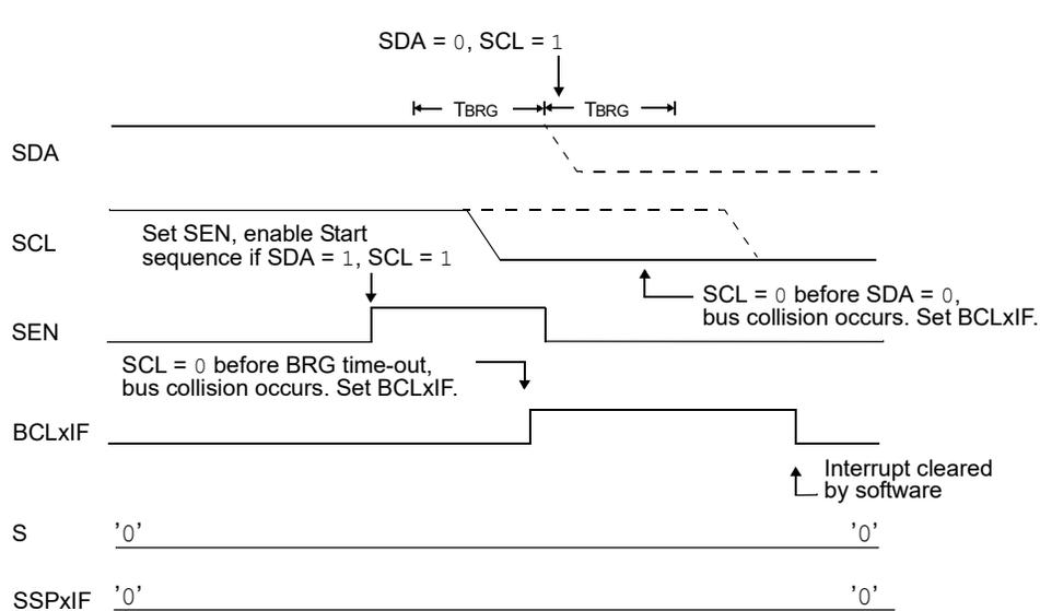
If the SDA pin is sampled low during this count, the BRG is reset and the SDA line is asserted early (Figure 29-35). If, however, a '1' is sampled on the SDA pin, the SDA pin is asserted low at the end of the BRG count. The Baud Rate
