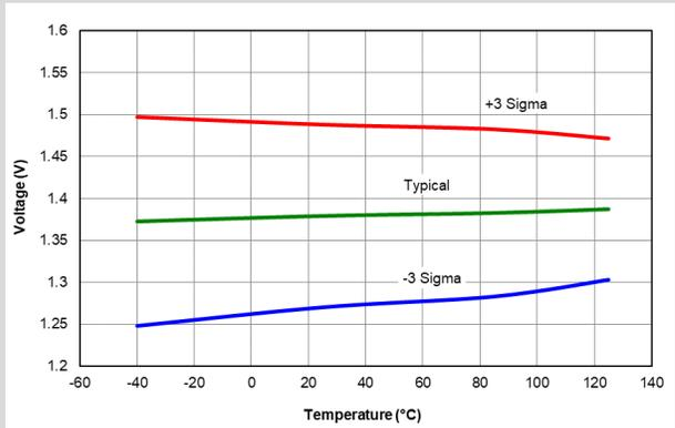
**Figure 40-105. POR REARM Voltage, Normal Power Mode, PIC16F18426/46 only**
