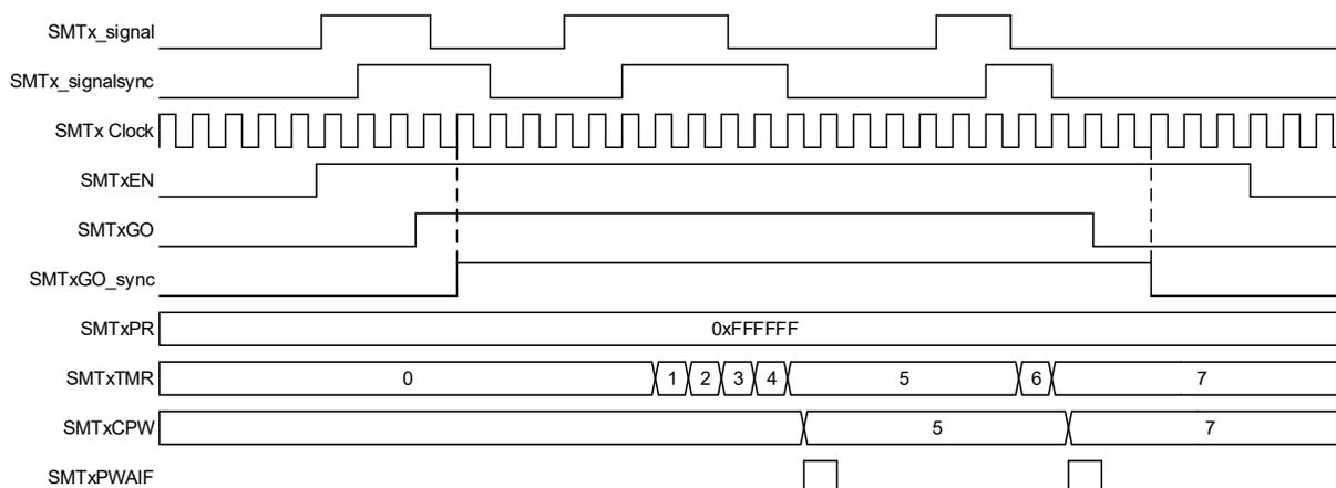
Figure 21-4. Gated Timer Mode, Single Acquisition Timing Diagram
