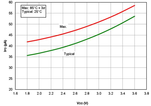
**Figure 40-5.  $I_{DD}$  Fixed Voltage Reference (FVR), PIC16F18426/46 only**
