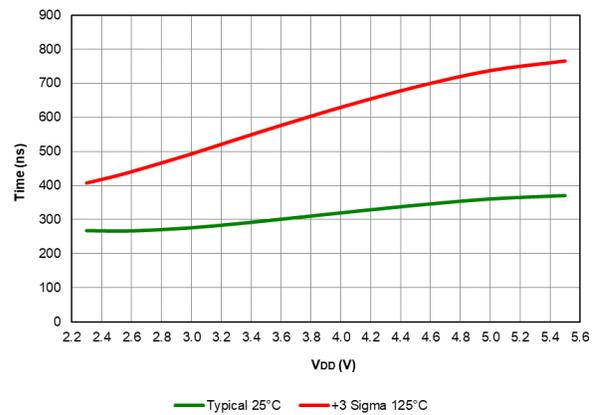
**Figure 40-89. Band Gap Ready Time, PIC16LF18426/46 only**
