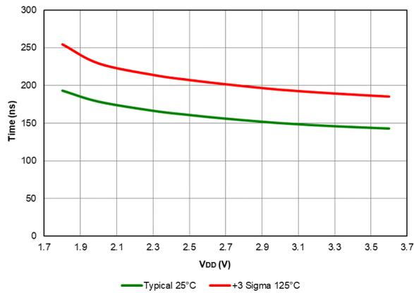
**Figure 40-86. Comparator Response Time Falling Edge, PIC16F18426/46 only**
