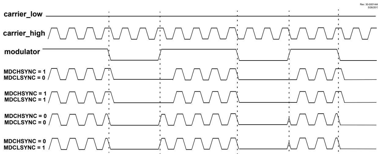
**Figure 27-3. No Synchronization (MDCHSYNC = 0, MDCLSYNC = 0)**
