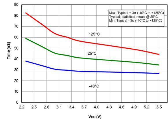
**Figure 40-85. Comparator Response Time Falling Edge, PIC16LF18426/46 only**
