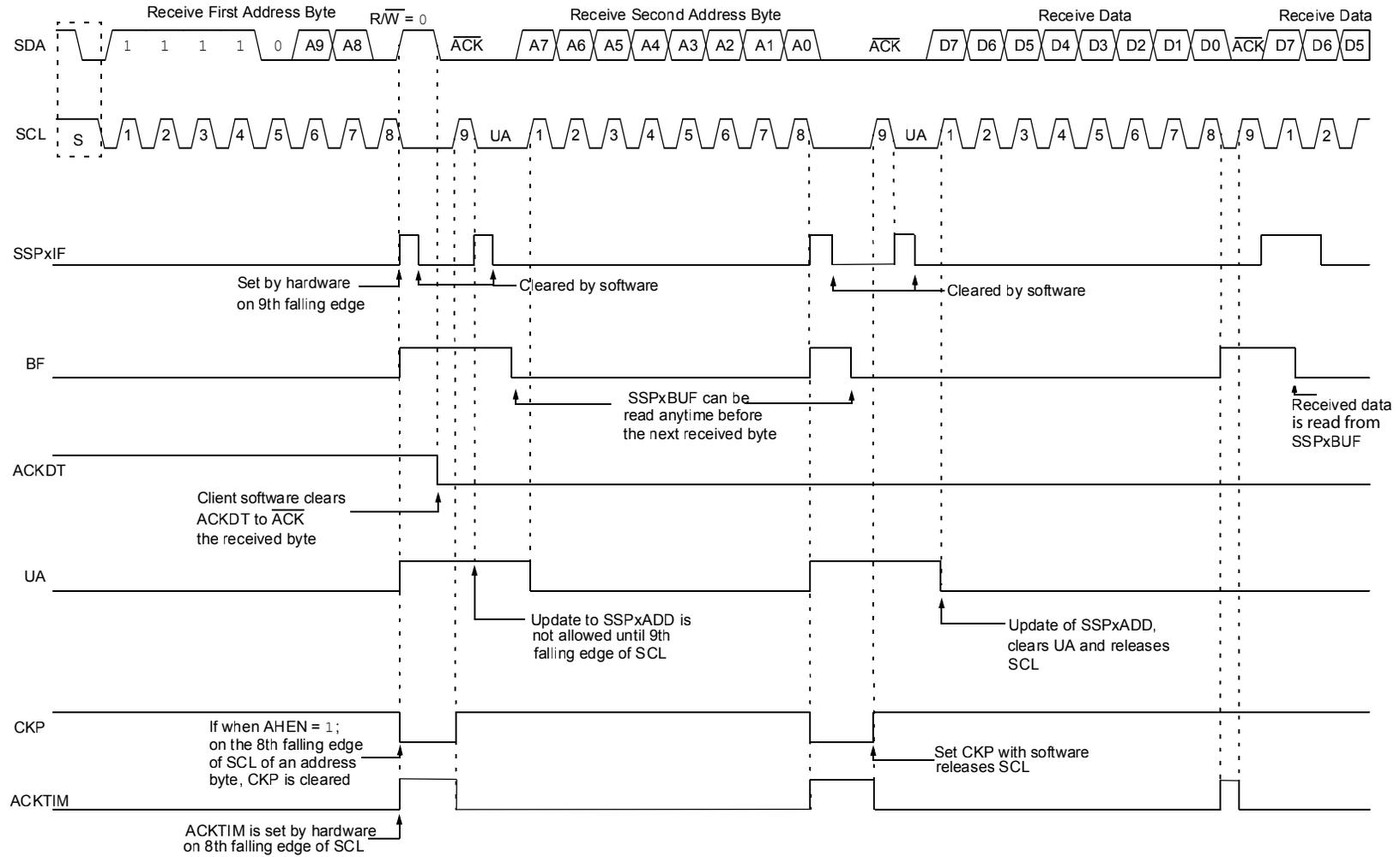
Figure 29-22. I<sup>2</sup>C Client, 10-Bit Address, Transmission (SEN = 0, AHEN = 0, DHEN = 0)
