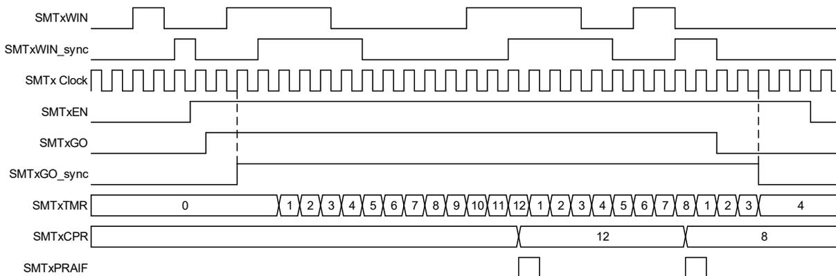
Figure 21-10. Windowed Measurement Mode, Single Acquisition Timing Diagram
