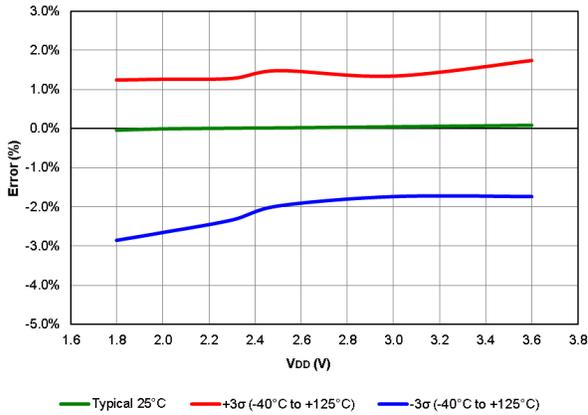
**Figure 40-28. HFINTOSC Typical Frequency Error, PIC16F18426/46 only**
