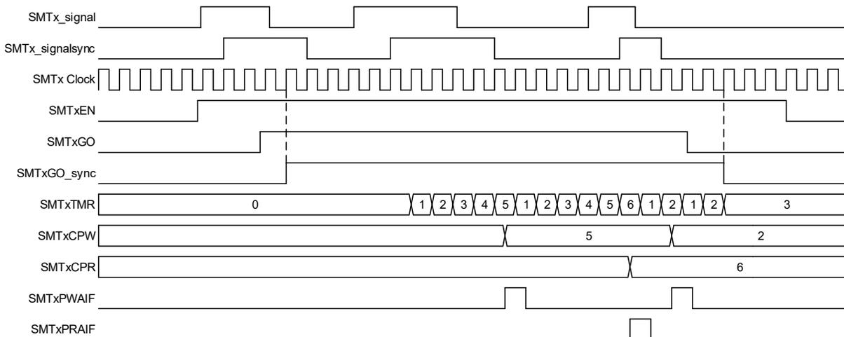
**Figure 21-8. High and Low Measurement Mode, Single Acquisition Timing Diagram**
