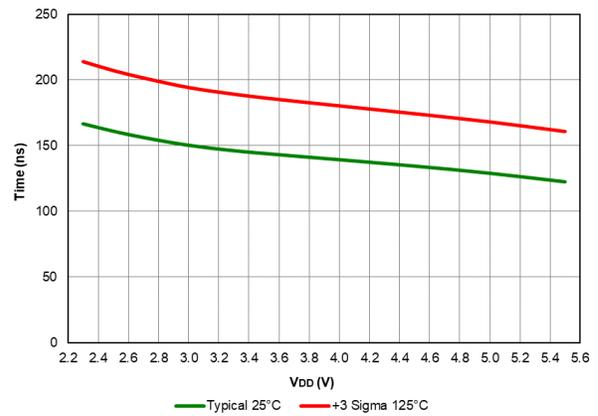
**Figure 40-87. Comparator Response Time Rising Edge, PIC16LF18426/46 only**
