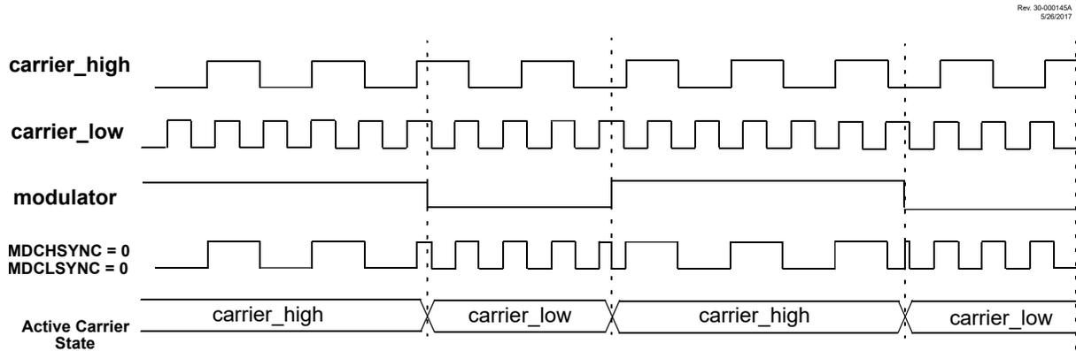
**Figure 27-4. Carrier High Synchronization (MDCHSYNC = 1, MDCLSYNC = 0)**
