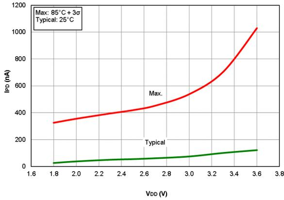
**Figure 40-2.  $I_{PD}$  Watchdog Timer (WDT), PIC16LF18426/46 only**
