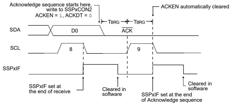
Note:  $T_{BRG}$  = one Baud Rate Generator period.
