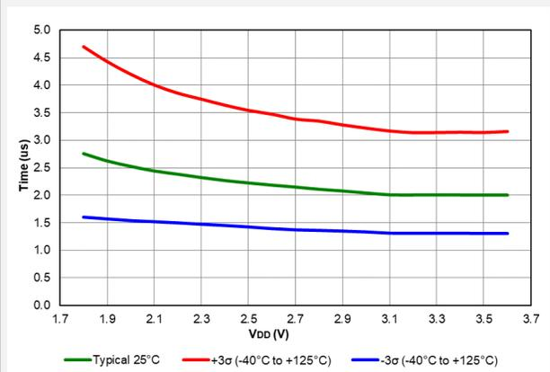
**Figure 40-67. ADC RC Oscillator Period, PIC16F18426/46 only**
