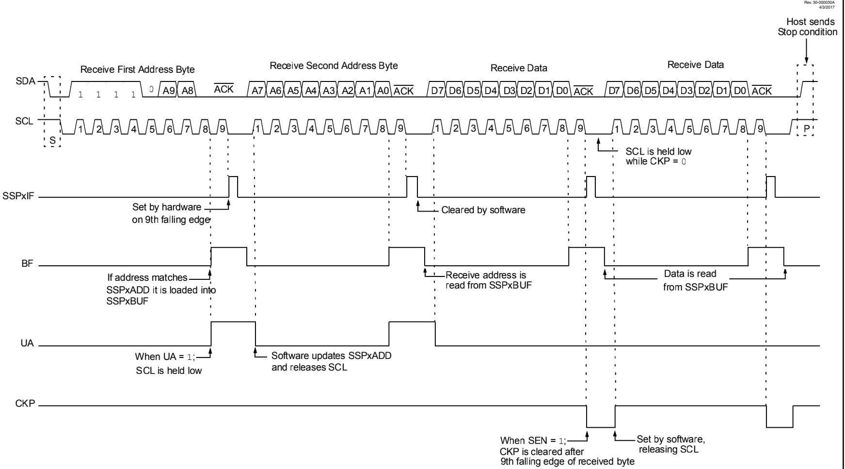
Figure 29-21. I<sup>2</sup>C Client, 10-Bit Address, Reception (SEN = 0, AHEN = 1, DHEN = 0)
