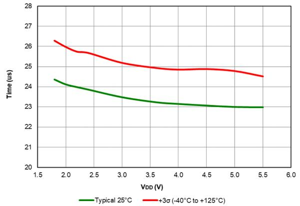
**Figure 40-111. Wake from Sleep, VREGPM = 1, HFINTOSC = 16 MHz, PIC16F18426/46 only**
