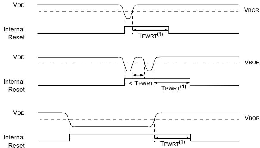
**Note:**  $T_{PWRT}$  delay only if the PWRTS bit field is programmed to a value different from '11'.
