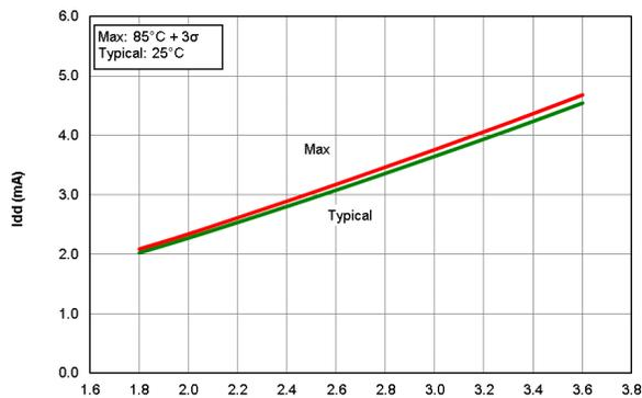
**Figure 40-16.  $I_{DD}$  HS Oscillator 32 MHz, PIC16F18426/46 only**
