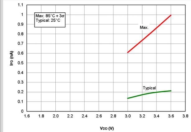
**Figure 40-9.  $I_{PD}$  Comparator, PIC16LF18426/46 only**
