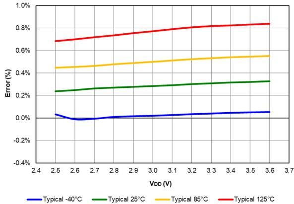
**Figure 40-94. FVR Voltage Error 2x, PIC16F18426/46 only**
