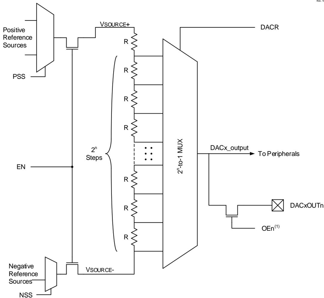
Note 1: The output enable bits are configured so that they act as a “one-hot” system, meaning only one DAC output can be enabled at a time.
