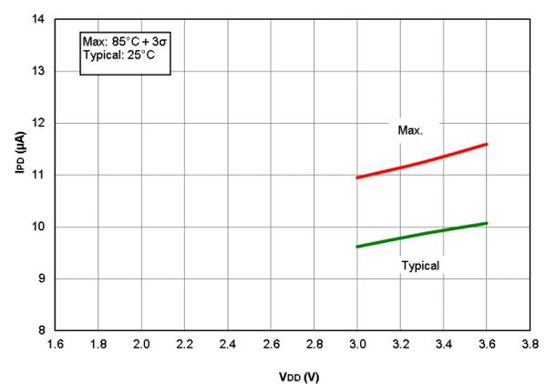
**Figure 40-7.  $I_{PD}$  Brown-Out Reset (BOR), BORV = 1, PIC16F18426/46 only**
