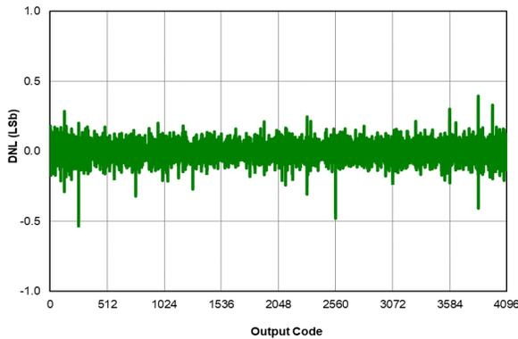
**Figure 40-50. ADC 12-Bit Mode, Single-Ended DNL,  $V_{DD} = 3.0V$ ,  $V_{REF} = 3.0V$ ,  $T_{AD} = 4 \mu s$ ,  $25^{\circ}C$ , All devices**
