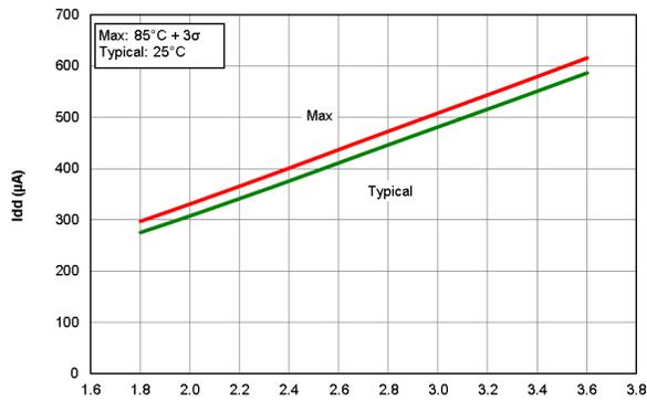
**Figure 40-14.  $I_{DD}$  XT Oscillator 4 MHz, PIC16F18426/46 only**
