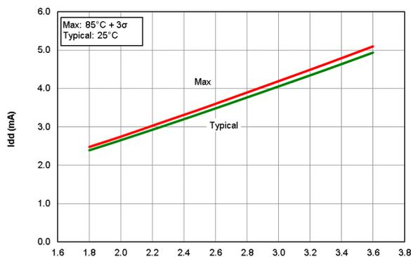
**Figure 40-18.  $I_{DD}$  HFINTOSC Mode,  $F_{OSC}$  = 32 MHz, PIC16F18426/46 only**
