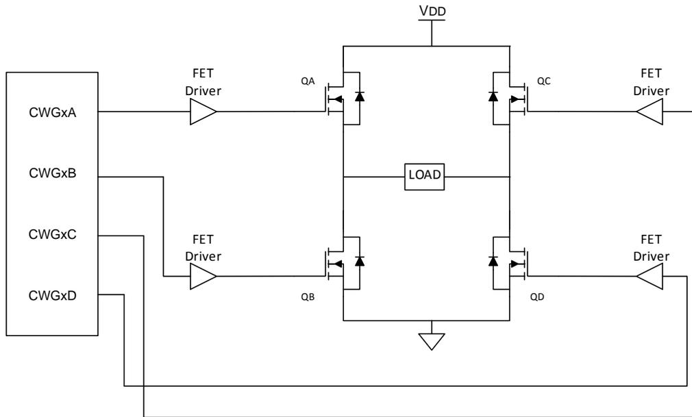
**Figure 25-6. Simplified CWG Block Diagram (Forward and Reverse Full-Bridge Modes)**
