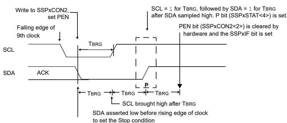
Note:  $T_{BRG}$  = one Baud Rate Generator period.
