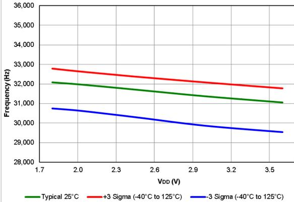
**Figure 40-26. LFINTOSC Frequency, PIC16F18426/46 only**
