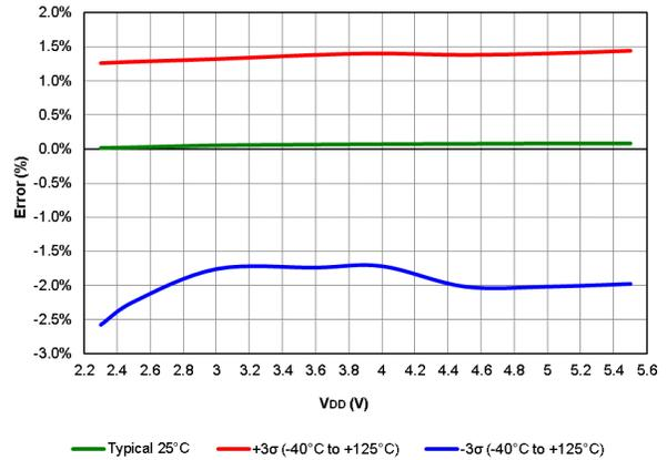
**Figure 40-29. HFINTOSC Frequency Error V<sub>DD</sub> = 3V, All devices**
