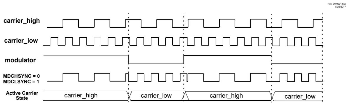
**Figure 27-6. Full Synchronization (MDCHSYNC = 1, MDCLSYNC = 1)**
