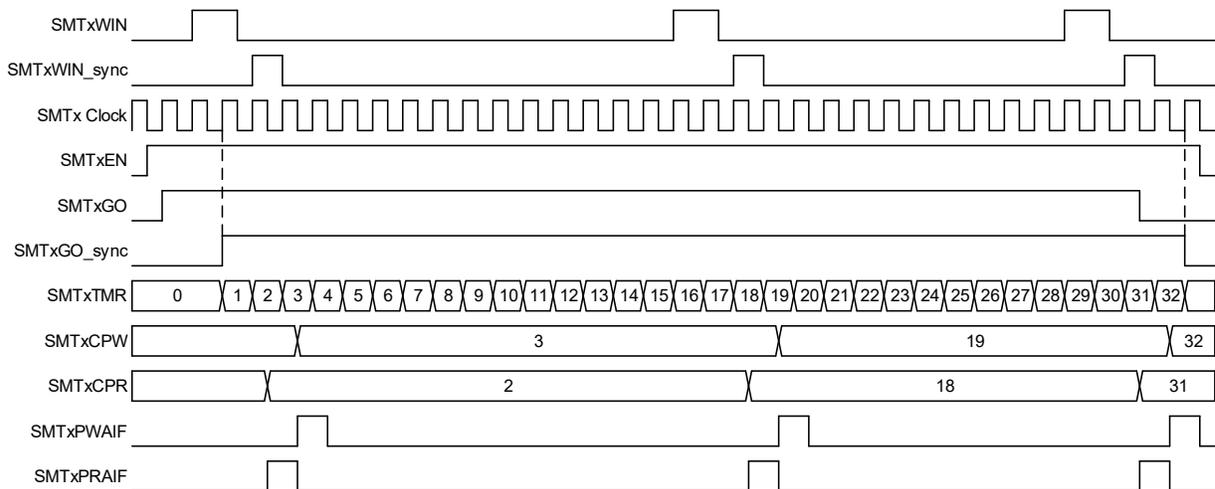
**Figure 21-16. Capture Mode, Single Acquisition Timing Diagram**
