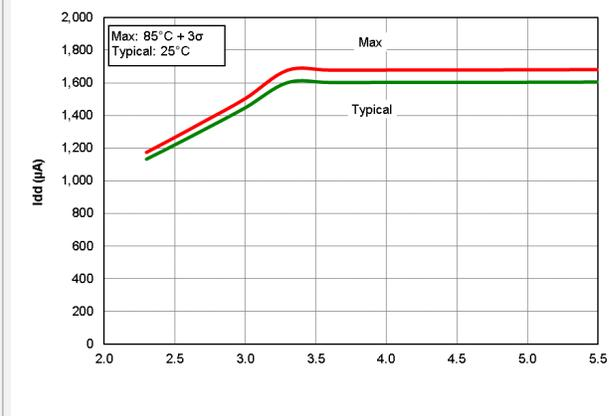
**Figure 40-23.  $I_{DD}$  HFINTOSC Doze Mode,  $F_{OSC} = 16$  MHz, PIC16LF18426/46 only**
