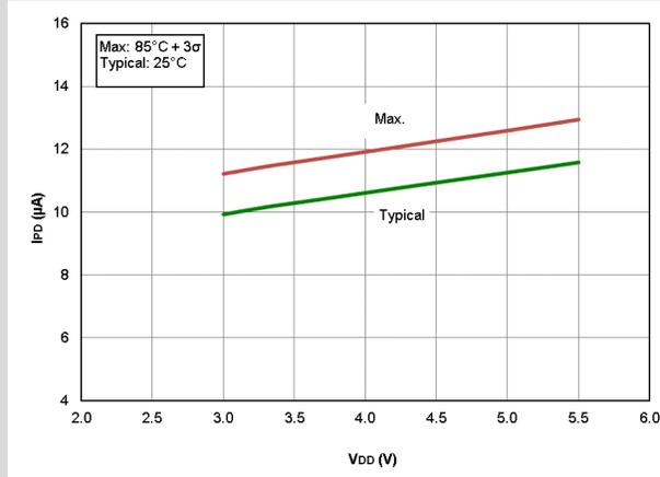
**Figure 40-8.  $I_{PD}$  Low-Power Brown-Out Reset, LPBOR = 0, PIC16LF18426/46 only**
