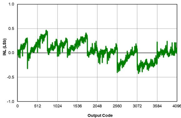
**Figure 40-52. ADC 12-Bit Mode, Single-Ended INL,  $V_{DD} = 3.0V$ ,  $V_{REF} = 3.0V$ ,  $T_{AD} = 1 \mu s$ ,  $25^{\circ}C$ , All devices**
