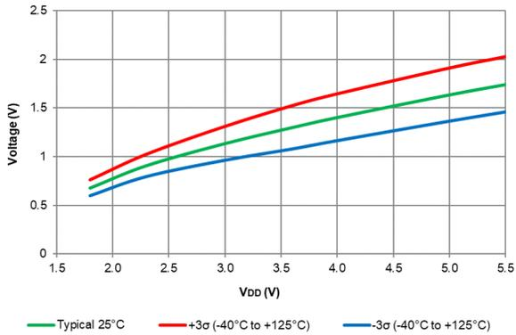
**Figure 40-98. Input Level TTL, All devices**
