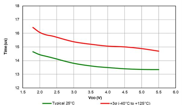
**Figure 40-109. Wake from Sleep, VREGPM = 1, HFINTOSC = 4 MHz, PIC16F18426/46 only**
