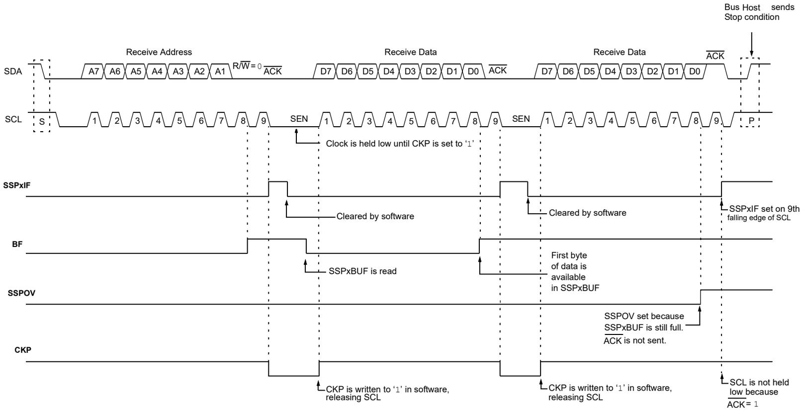
Figure 29-16. I<sup>2</sup>C Client, 7-Bit Address, Reception (SEN = 0, AHEN = 1, DHEN = 1)
