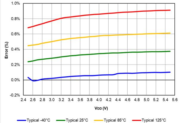
**Figure 40-95. FVR Voltage Error 4x, PIC16F18426/46 only**
