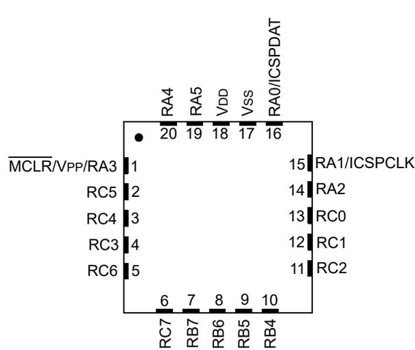
**Note:** It is recommended that the exposed bottom pad be connected to V<sub>SS</sub>.
