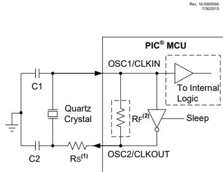
Figure 8-4. Ceramic Resonator Operation (XT or HS Mode)
