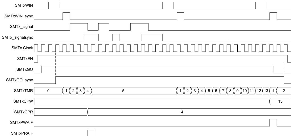
**Figure 21-14. Time of Flight Mode, Single Acquisition Timing Diagram**
