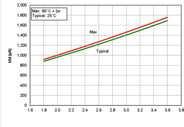
**Figure 40-22.  $I_{DD}$  HFINTOSC Idle Mode,  $F_{OSC} = 16$  MHz, PIC16F18426/46 only**
