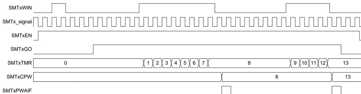
**Figure 21-19. Gated Counter Mode, Single Acquisition Timing Diagram**
