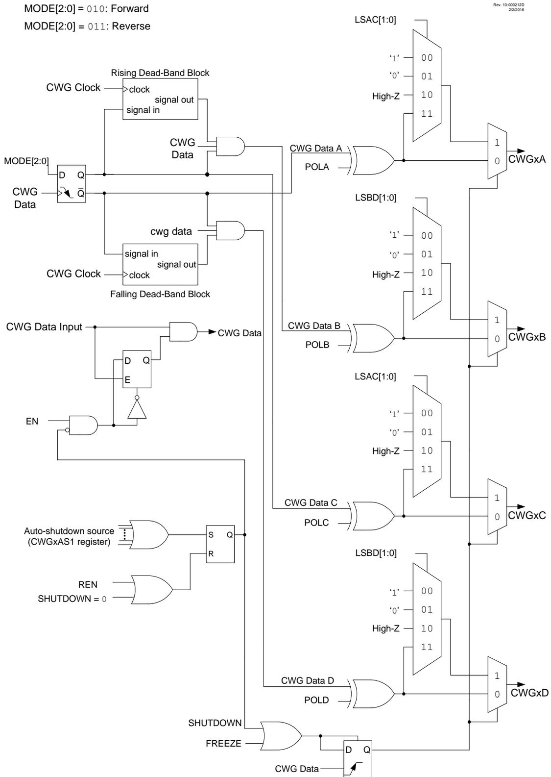
In Forward Full-Bridge mode (**MODE** = 010), CWGxA is driven to its Active state, CWGxB and CWGxC are driven to their Inactive state, and CWGxD is modulated by the input signal, as shown in [Figure 25-7](#).
