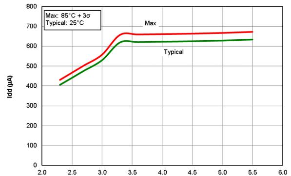
**Figure 40-15.  $I_{DD}$  HS Oscillator 32 MHz, PIC16LF18426/46 only**
