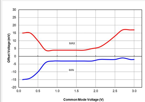
**Figure 40-79. Comparator Offset, Normal Power Mode (CxSP = 1), V<sub>DD</sub> = 3.0V, Typical Measured Values from -40°C to 125°C, All devices**
