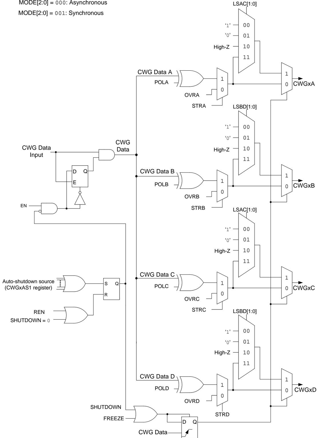
For example, when **STRA** = 0, the corresponding pin is held at the level defined by **OVRA**. When **STRA** = 1, the pin is driven by the modulated input signal.
