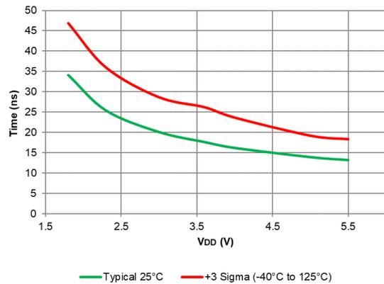
**Figure 40-100. Fall Time, Slew Rate Control Enabled, All devices**
