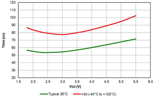
**Figure 40-110. Wake from Sleep, VREGPM = 0, HFINTOSC = 16 MHz, PIC16F18426/46 only**
