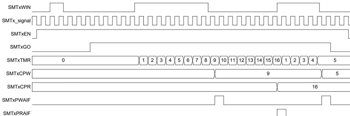
**Figure 21-21. Windowed Counter Mode, Single Acquisition Timing Diagram**
