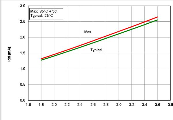
**Figure 40-20.  $I_{DD}$  HFINTOSC Mode,  $F_{OSC} = 16$  MHz, PIC16F18426/46 only**
