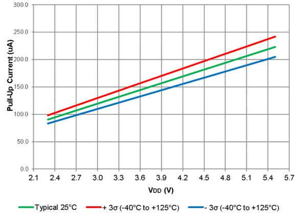
**Figure 40-31. Weak Pull-Up Current, PIC16LF18426/46 only**
