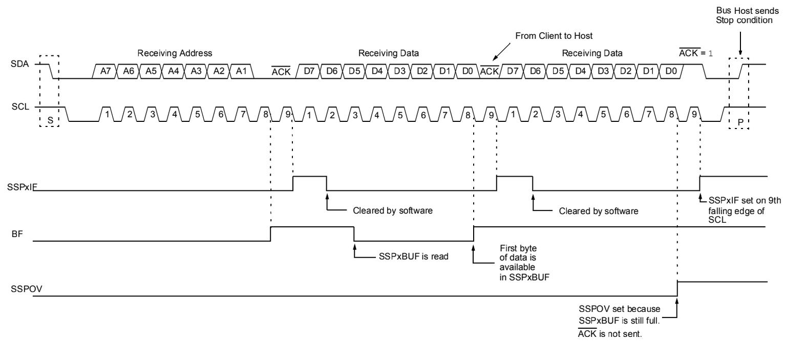
Figure 29-15. I<sup>2</sup>C Client, 7-Bit Address, Reception (SEN = 1, AHEN = 0, DHEN = 0)
