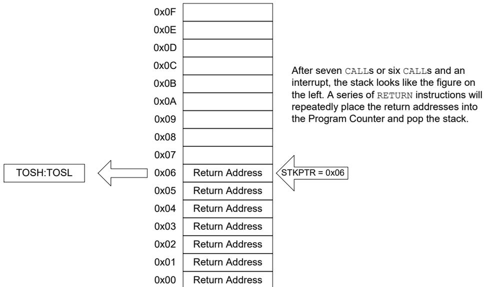
Figure 5-7. Accessing the Stack Example 4
