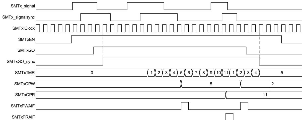
**Figure 21-6. Period and Duty Cycle, Single Acquisition Mode Timing Diagram**
