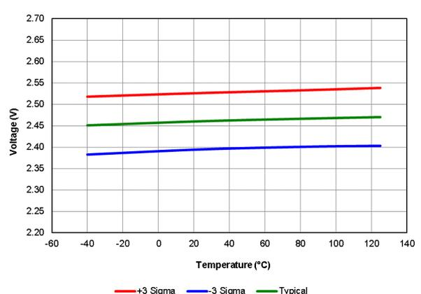
**Figure 40-43. Brown-Out Reset Hysteresis, Trip Point BORV = 01, PIC16F18426/46 only**
