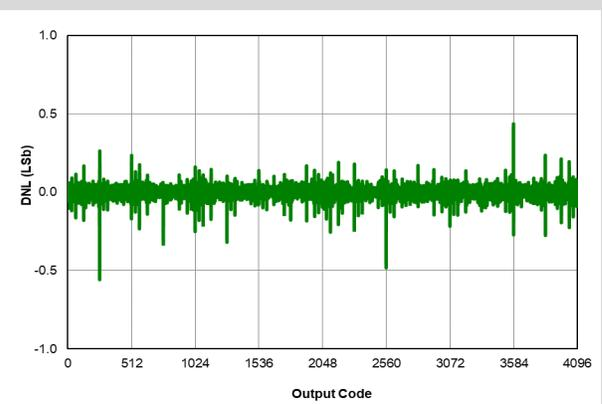
**Figure 40-49. ADC 12-Bit Mode, Single-Ended DNL,  $V_{DD} = 3.0V$ ,  $V_{REF} = 3.0V$ ,  $T_{AD} = 1 \mu s$ ,  $25^{\circ}C$ , All devices**
