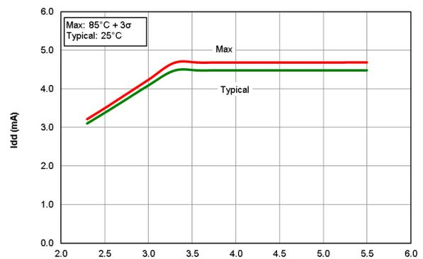
**Figure 40-19.  $I_{DD}$  HFINTOSC Mode,  $F_{OSC} = 16$  MHz, PIC16LF18426/46 only**
