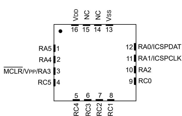
**Note:** It is recommended that the exposed bottom pad be connected to  $V_{SS}$ .
