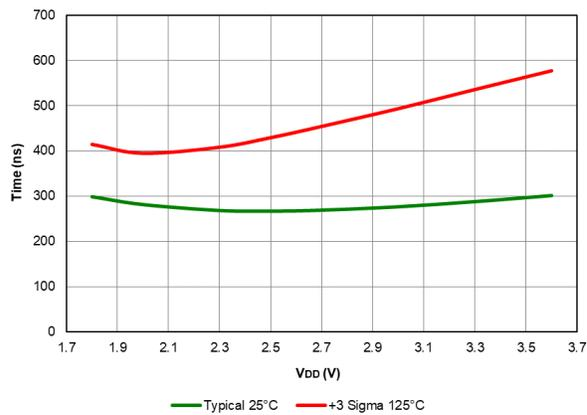
**Figure 40-88. Comparator Response Time Rising Edge, PIC16F18426/46 only**
