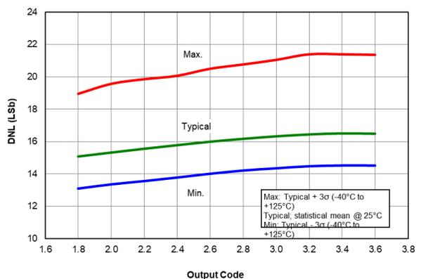
**Figure 40-73. Absolute Value of DAC DNL Error,  $V_{DD} = 3.0V$ ,  $V_{REF} = V_{DD}$ , All devices**
