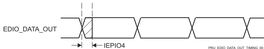
Figure 7-101. PRU_ICSSG IEP Digital IOs Timing Requirements
