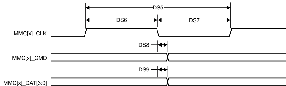
Figure 7-66. MMC1 – Default Speed – Transmit Mode
