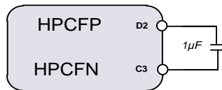
Figure 39: Charge Pump Flying Capacitor
