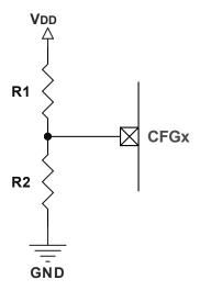
Note: It is recommended that R1 and R2 be greater than 100  $k\Omega$  for lower power consumption.
