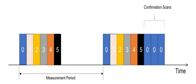
Figure 7-3. Confirmation Scan for Multiple Channels
