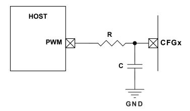
**Note:** Refer to Microchip Application Note TB3250, "Using PWM to Generate Analog Output" (DS90003250), for details on choosing the appropriate values of R and C.
