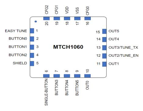
**Note:** Connecting the exposed bottom pad to  $V_{SS}$  is recommended. However, it must not be the only  $V_{SS}$  connection to the device.
