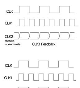
Using CLK1 as feedback will always result in synchronized rising edges between ICLK and CLK1 if CLK1 is used as feedback. CLK2 could be a falling edge compared to ICLK. Therefore, wherever possible, it is recommended to use CLK2 for feedback, which will synchronize the rising edges of all three clocks.
