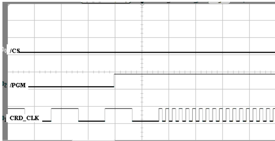
Figure 28. Clock Divider Timing Details
