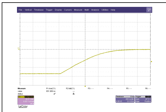
FIGURE 1-6: Typical HV_{OUT} from -135V to 0V, Load = 100pF
